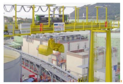
4 Off-standard LNG hoists from STAHL CraneSystems are used for maintenance work on the pumps in liquefied gas tanks. The wire rope hoists are equipped with two separately driven rope drums with 2,400 kg S.W.L. each. An additional small slewing crane is equipped with an SH30 Ex wire rope hoist and used as an auxiliary crane for transporting tools and components onto the tank's platform.
